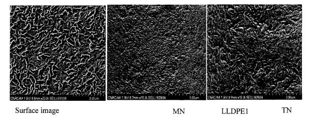
Figure 5.2. Comparison between surface and bulk morphologies of different PE films (MD $\uparrow$ , TD $\rightarrow$ ).
