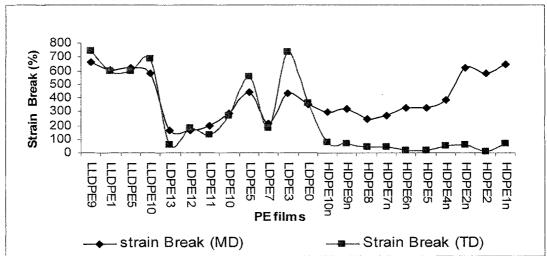
Figure 4.11. Measured mechanical properties.
