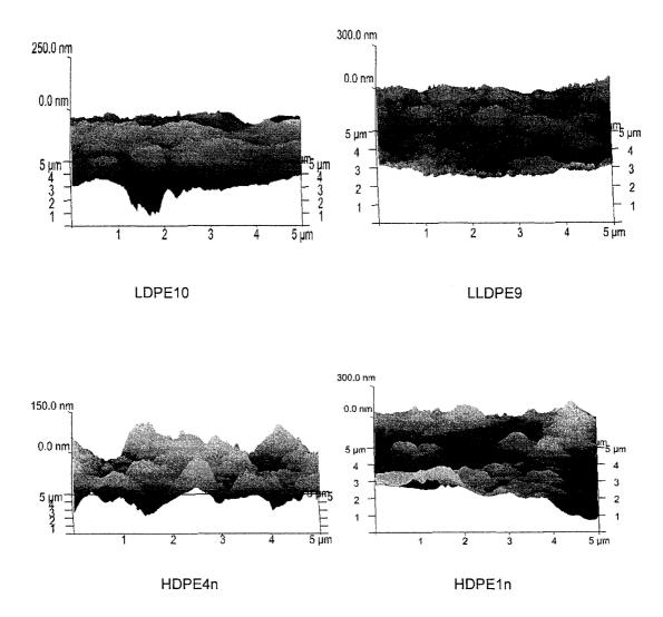
Figure 4.4. 3D surface plot analysis of AFM height images of blown films.
