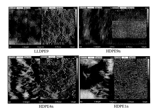
Figure 4.3. AFM images of the surfaces of blown films.
