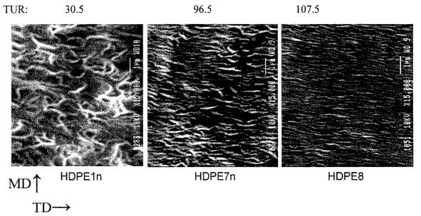
Figure 5.3. Morphological characteristics of PE films with different structure using SEM.
