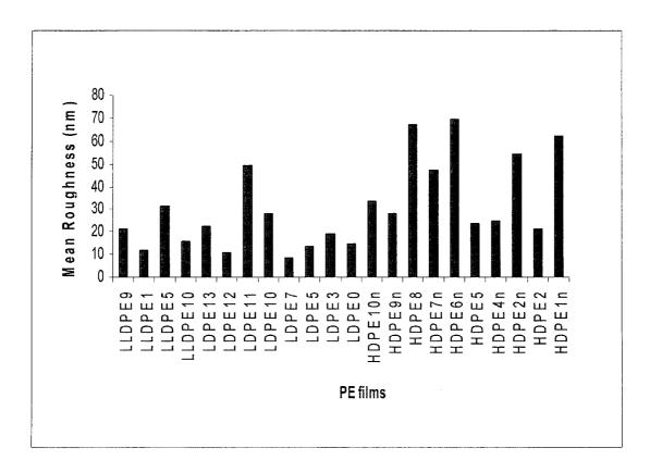
Figure 4.5. The surface roughness of the samples measured by AFM.
