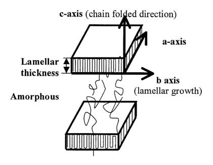
FIG 6.7. The folded chain mode in PE
