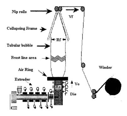
Figure 1.1. A schematic illustration of the blown film process
