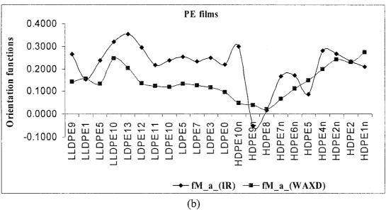
Figure 4.8. Measured orientation functions from two FTIR and WAXD techniques: (a) Orientation factors of crystalline b-axis in MD; (b) Orientation factors of crystalline a-axis in MD; (c) Orientation factors of crystalline b-axis in TD; (d) Orientation factors of crystalline a-axis in TD; (e) Orientation factors of amorphous phase in MD; and (f) Orientation factors of amorphous phase in TD.
