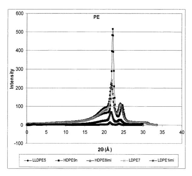
FIG. 6.1. WAXS profiles for PE blown films
