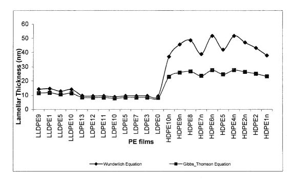
Figure 4.10. Measured lamellar thickness from two different equations.
