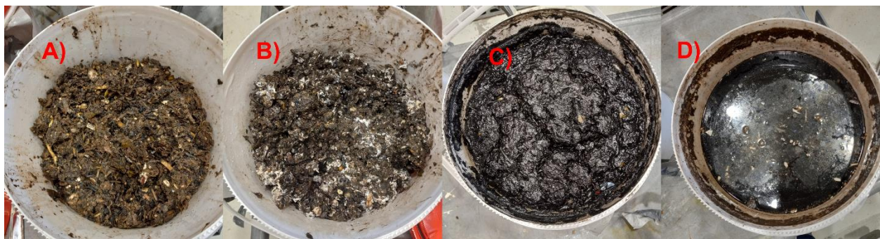
Figure S2: Pictures of the samples from AD plant 2. a) Light rejects (LR2); b) Heavy rejects (HR2); c) Digestate (D2); d) Food waste (FW2).
