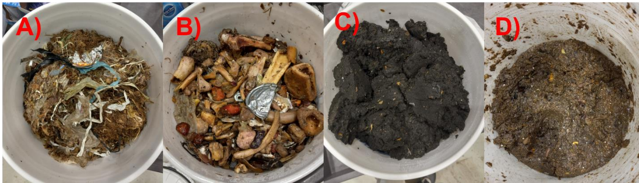
Figure S1: Pictures of the samples from AD plant 1. a) Light rejects (LR1); b) Heavy rejects (HR1); c) Digestate (D1); d) Food waste (FW1).
