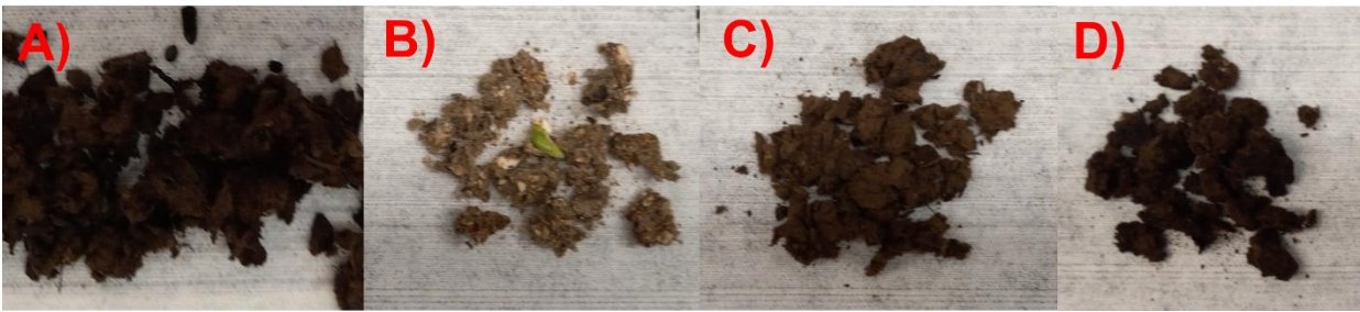
Figure S4: Pictures of the hydrochars from AD plant 2. a) Light rejects (H-LR2); b) Heavy rejects (H-HR2); c) Digestate (H-D2); d) Food waste (H-FW2).
