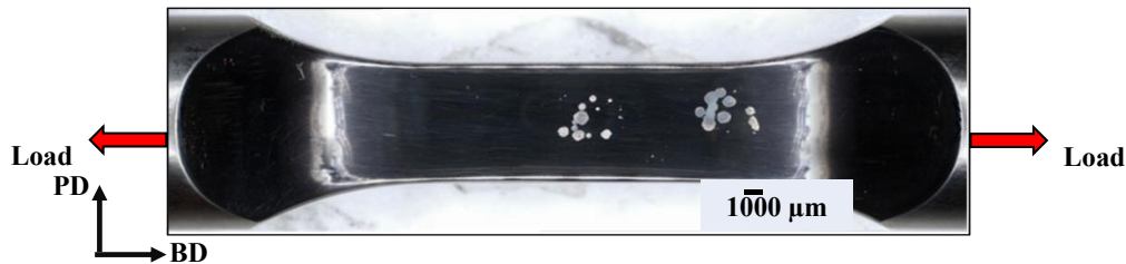
Figure 3-5. Representative FC specimen after electrochemical pitting.
