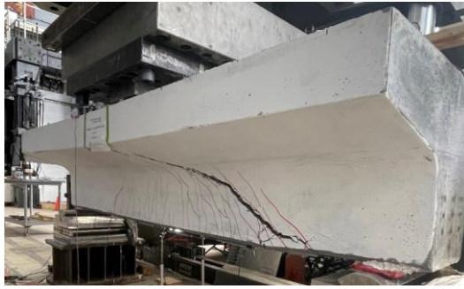
a) After bending test
