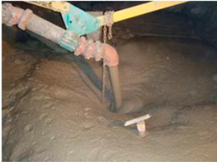
Figure 2-23 Example of cemented paste backfill in an underground mine in Peru (reproduced of Cacciuttolo & Marinovic 2023 with permission)
