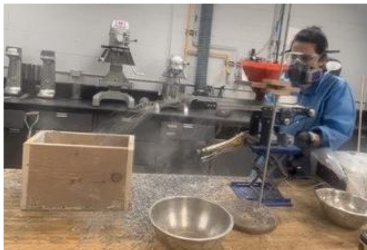
Figure 4-3 Distribution of waste rock into the mold using the slinger system
