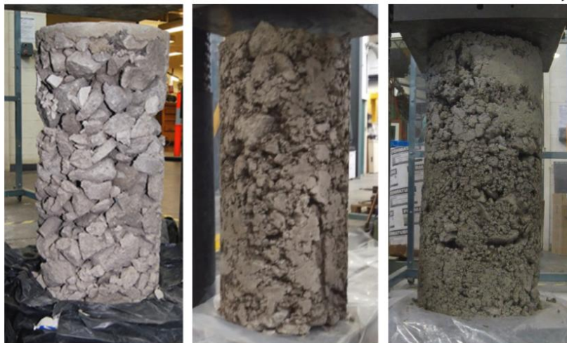
Figure 2-24 Laboratory-produced rockfill samples (reproduced of Sainsbury et al. 2021 with permission)
