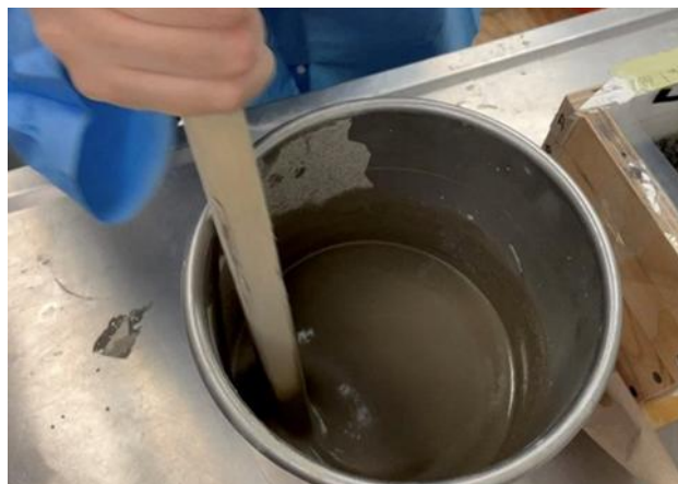
Figure 3-4 Manual mixing of the paste backfill
