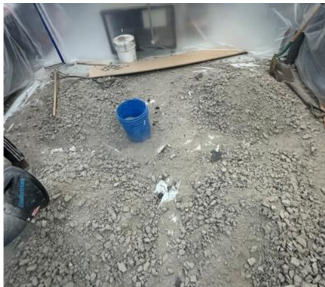
Figure 3-19 Waste rock of underground mine A used for the large-scale tests
