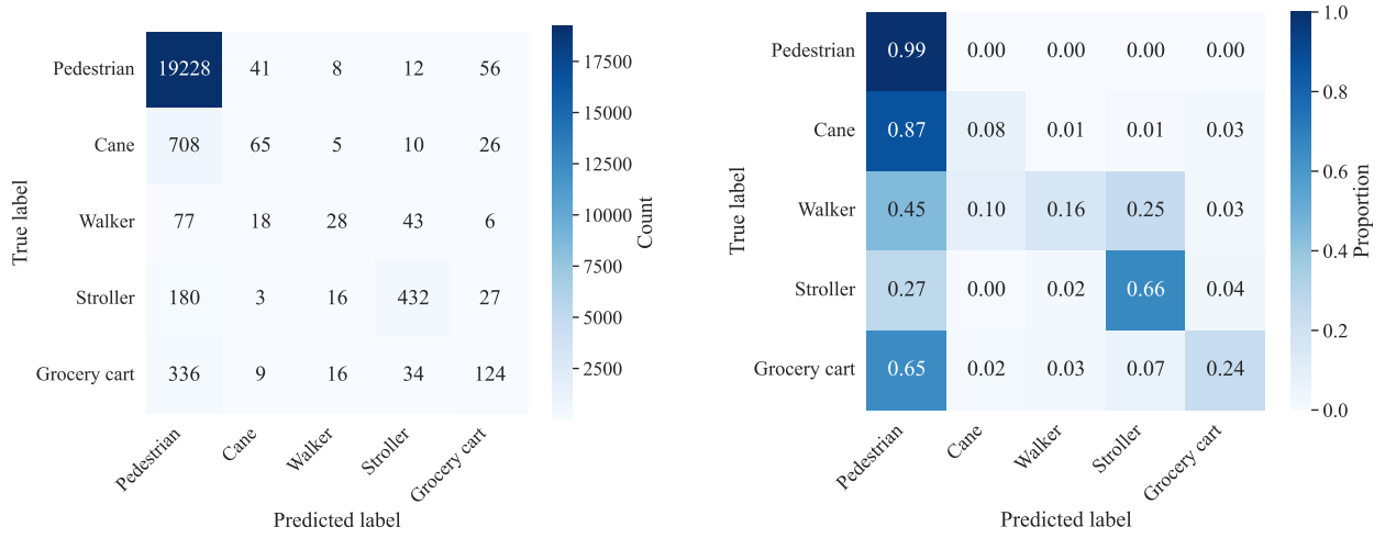
Figure 7.5 Confusion matrix of YOLOv11 for pedestrian categories. The left figure presents the confusion matrix as raw counts, while the right shows the row-wise normalized matrix; in both cases, rows correspond to ground-truth labels and columns to predicted labels. Pedestrian refers to the pedestrians without AWDs.
