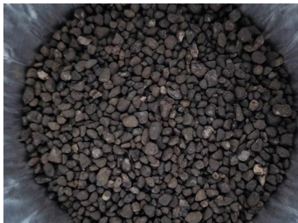
Figure B.3: Photo of a media sample taken from the top of the cored biofilter
