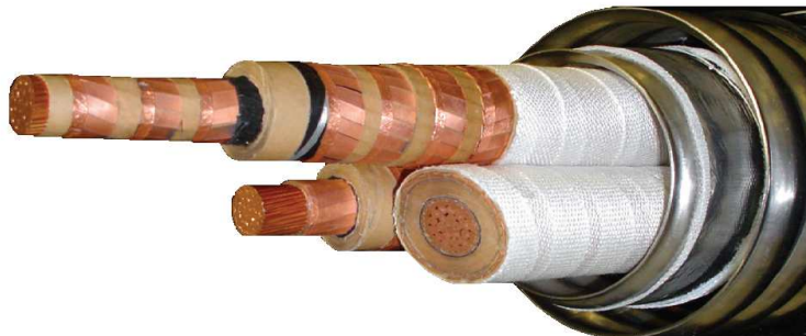
Figure 2.10 An HTS cable with the Triad design. In this design, three identical single phase cables are put together in a common cryostat.
