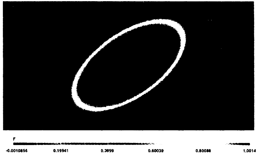
Figure 7.3 Deformation of a single viscoelastic drop in a Newtonian matrix ( Ca = 10 ), after 30 time steps
