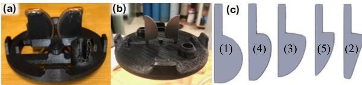
Figure 4.9 Prototype development steps for a gliding arc; a) Initial copper electrodes prototype; b) replacement of electrodes for stainless steel; c) various electrode geometries studied along with reactor b) design. The numbers correspond to the electrode shape as found in figure 4.10.
