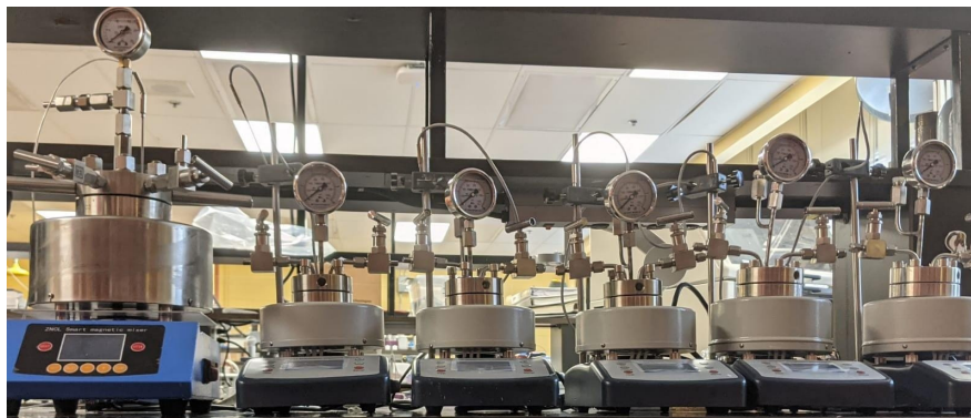
Figure 4.1 Multi scale lab reactors. From left to right: 250 mL ( R_{250} ), 3 \times 25 mL ( R_{25} ), and 2 \times 50 mL ( R_{50} ).
