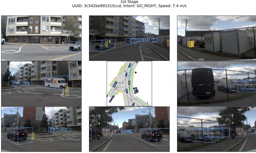
Figure 7.2 Driving Environment Overview Example scene of the driving problem and the context the agent is presented with. The agent does not perceive privileged information, i.e., the bounding boxes in the images and the vectorized scene representation in the center are only provided for illustrative purposes. In our experiments, the agent is limited to only observing the three front views, due to computational limitations, along with its speed and intention as textual prompts.
