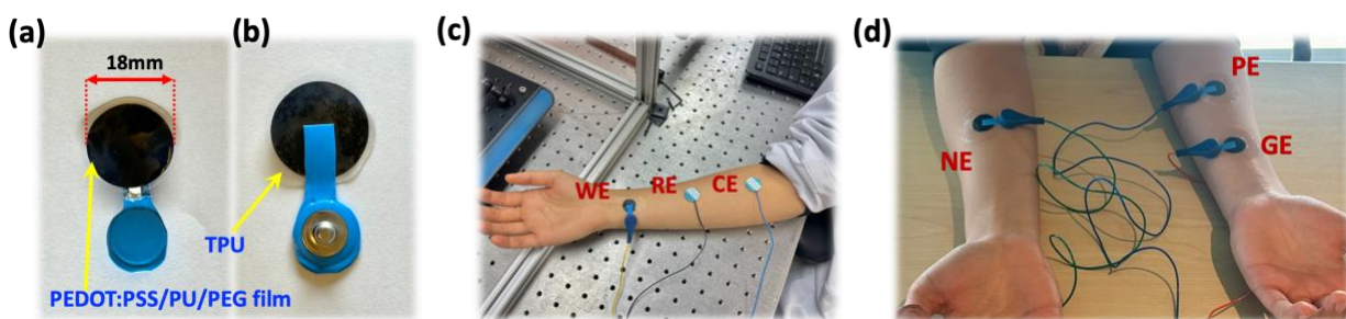
Figure S10. Electrode configuration and measurement setup. (a,b) Front and back views of the electrodes. (c) Photograph of the skin–electrode impedance and ECG measurement configuration. The PEDOT:PSS/PU/PEG film served as the working electrode (WE), while commercial Ag/AgCl gel electrodes (Natus®) were used as the reference (RE) and counter (CE) electrodes. Measurements were conducted on the same volunteer and at the same location. Skin–electrode impedance data are presented as mean \pm standard deviation ( n = 3 ). (d) ECG measurement configuration on a volunteer, showing the positive (PE) and ground (GE) electrodes positioned on the left forearm and the negative electrode (NE) on the right forearm.
