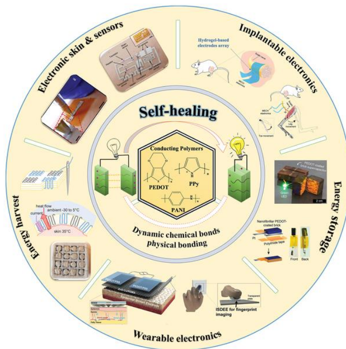
Figure 12. Schematic overview of representative applications of self-healing conductive polymers. By combining intrinsic conductivity with autonomous damage recovery, these materials support durable operation in electronic skin and sensors, implantable electronics, energy devices, and wearable systems [21].
