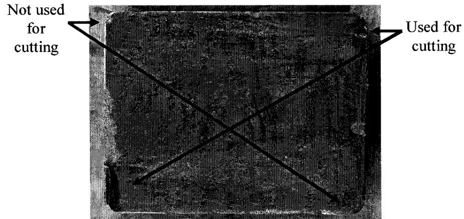
Figure 6.17. The other free corners of the square insert may be worn by chip even if not directly involve in cutting.
