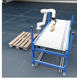
(a) Manipulator with suction gripper (b) Manipulator with parallel gripper
