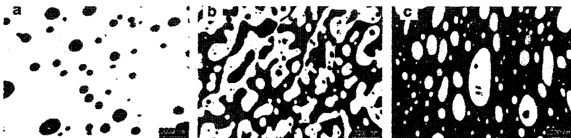
Figure 2.5: Transmission electron micrographs for PMMA/PS blends at different blend compositions: (a) 90/10, (b) 50/50, (c) 30/70 (Steinmann et al. (2001))
