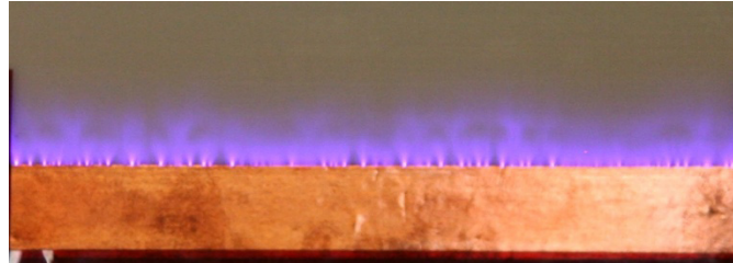
(a) 10.17 kV rms , straight electrode
