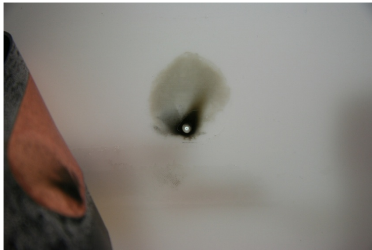
Figure 5.3: Teflon damage due to arc formation
