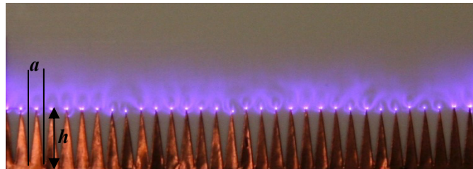
(c) 10.15 kV rms , serrated electrode
