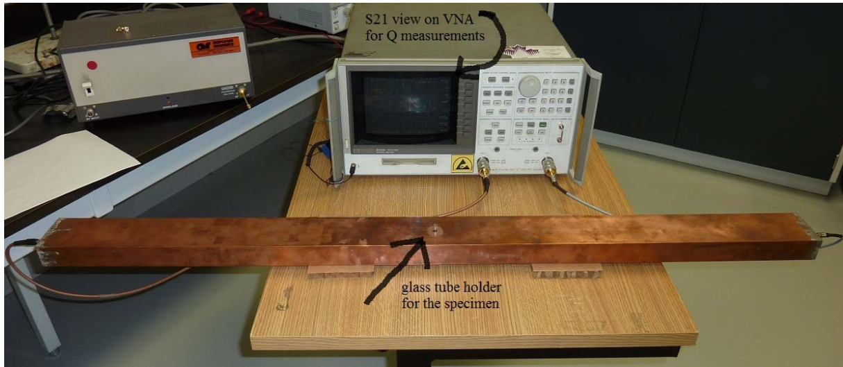
Figure 3-1: The cavity resonator built for our study at École Polytechnique de Montréal laboratories (the length of 1186.55 mm, and made of copper)
