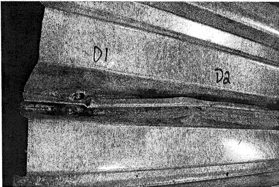
Figure 4.128. Weld failure at D1 (north), and sheet buckling at D2
