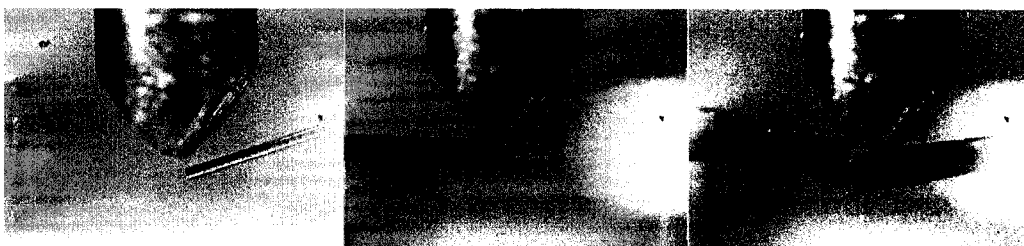
Figure 5.18: Fiber fracturing. Left: 0.5 W, 800 mbar, D = 77.9 \mu\text{m} , Center: 1.0 W, 275 mbar, D = 181.32 \mu\text{m} , Right: 2 W, 1000 mbar, D = 243.1 \mu\text{m}
