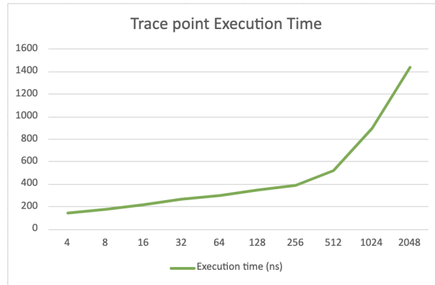
Figure 4.4 Result of trace point execution time benchmark
