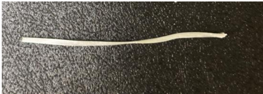
Figure 3.2 : Photo of a Polypropylene fiber used in this study for fiber reinforced CPB
