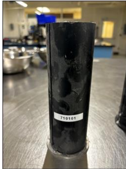
Figure 3.7 : A photo of ABS cylindrical mold for the UCS tests
