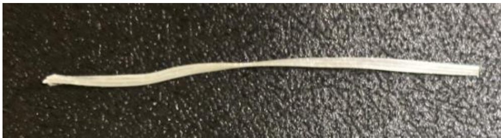
Figure 4.2 : Polypropylene fiber used in this study to make fiber reinforced CPB
