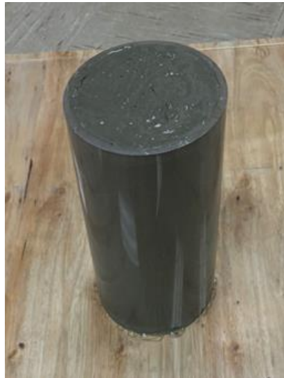
Figure 3.5 : A photo of the Plexiglas mold and backfill before slump test
