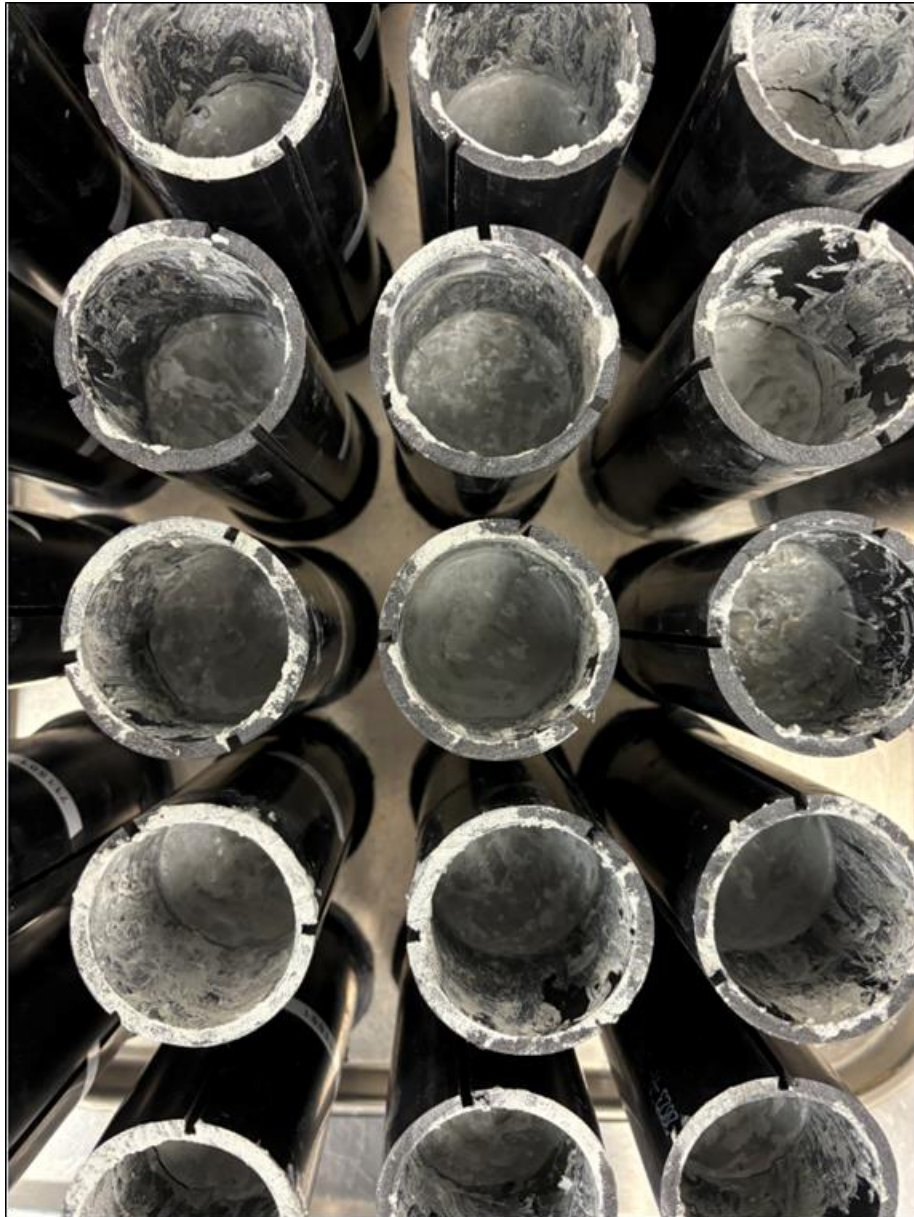
Figure 3.10 : Picture of unreinforced and fiber reinforced CPB during curing process
