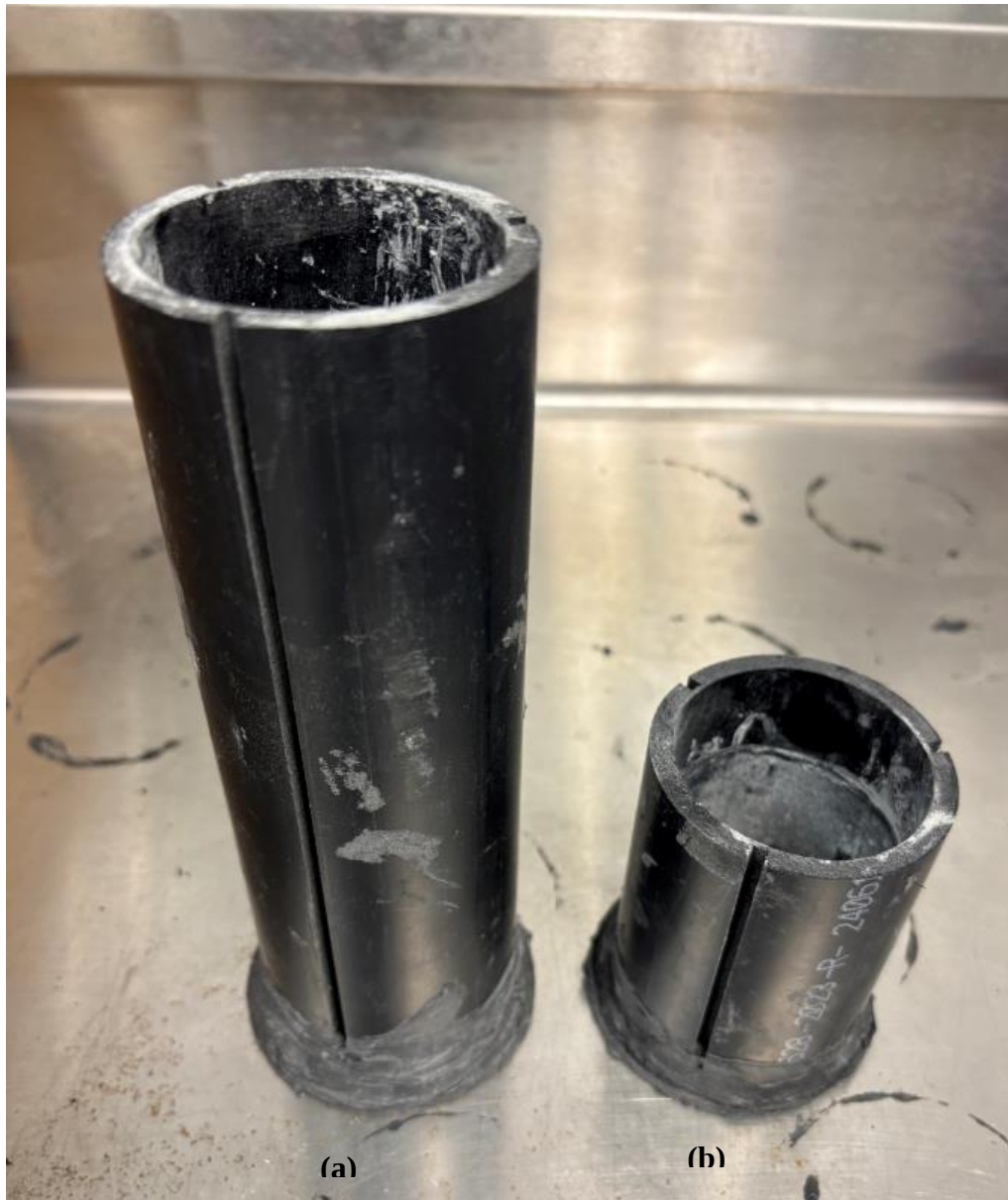
Figure 5.4 : Photos of ABS cylindrical molds for UCS (a) and STS (b) tests
