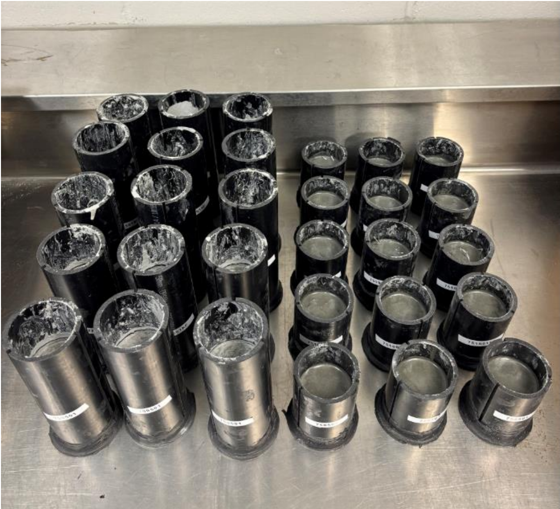
Figure 5.6 : Picture of unreinforced and fiber reinforced CPB during curing process, 6 days for UCS samples and 1 day for STS samples
