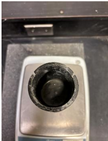
Figure 3.9 : Appearance of bleeding water after 2 minutes of manual vibration
