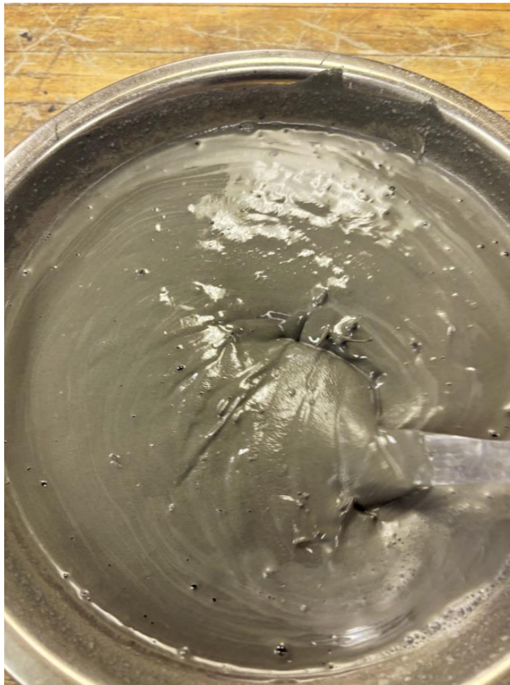
Figure 4.3 : A mixture with a solids content of at 65%, cement content of 5%, and fibers content of 0.5%
