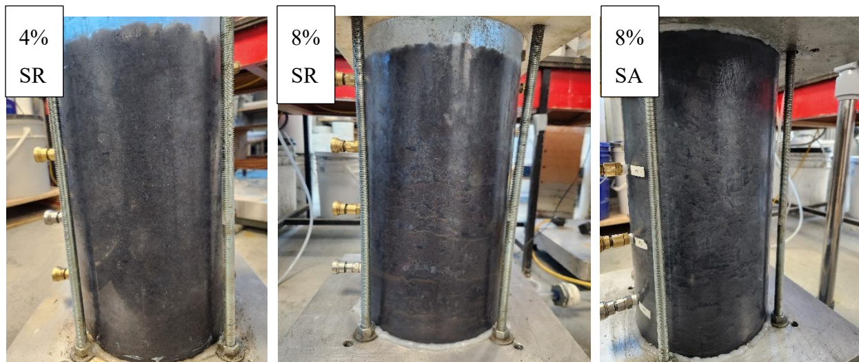
Figure 6.6: Post-compaction appearance of SA and SR materials at different water contents (4% vs. 8%).
