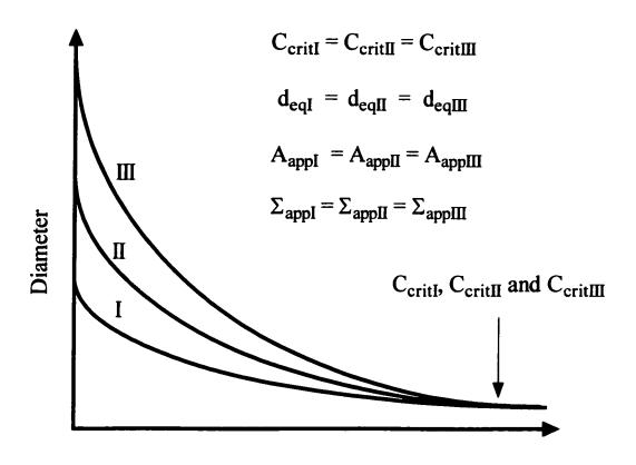
Figure 6.1b. Family of emulsification curves expected for a system in which all the modifier migrates to the interface and the modifier entirely suppresses dynamic coalescence.
