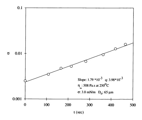
Figure 7 Relative distortion amplitude for PA thread containing SEBS-g-MA copolymer imbeded in a PS matrix
