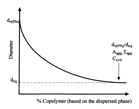
Figure 6.1a General features of an emulsification curve
