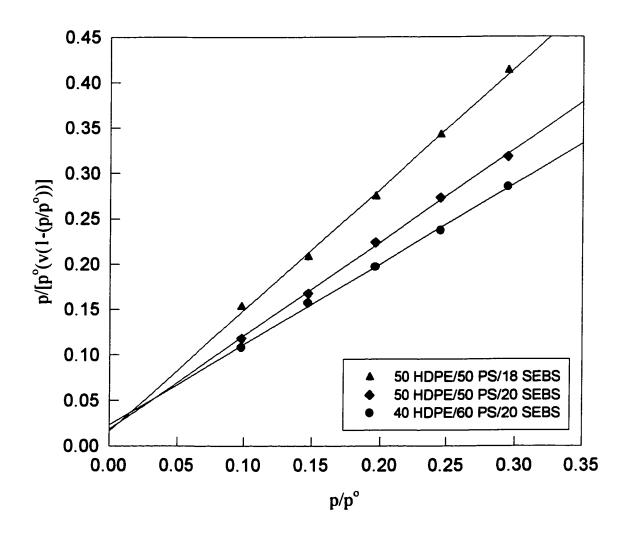
Figure 4.1. BET multiple point method for the extracted ternary blend systems.
