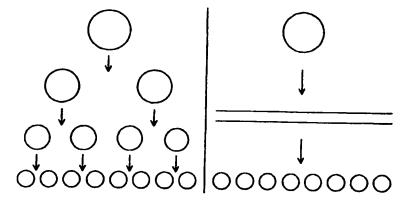
Figure 2. 2 Schematic presentation of the two dispersion mechanisms: on the left, the stepwise equilibrium mechanism of repeated breakup at Ca<sub>crit</sub>, and on the right, the transient mechanism of thread breakup during extension. (Janssen and Meijer, 1993)
