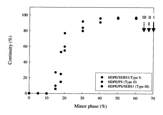
Figure 5.6 (a) Schematic illustration of continuity and dual phase continuity development for three different blend systems. I: compatible binary system, II: non-compatible binary blend system and III: compatible ternary system. The arrows stand for the disintegration points for three blend systems during extraction. HDPE/SEBS1 disintegrates at 70% PS (solid arrow), HDPE/PS at 68% PS (thick dash arrow) and HDPE/PS/SEBS1 at 66% PS (fine dash arrow).
