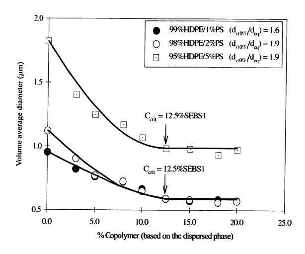
Figure 6.3a. A family of emulsification curves for 99%HDPE/1%PS, 98%HDPE/2%PS and 95%HDPE/5%PS blends.
