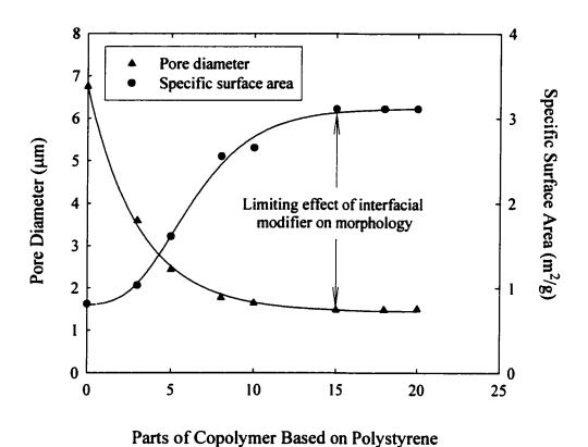
Figure 4.6. Effect of copolymer compatibilizer concentration on the specific surface area and pore size of extracted co-continuous blends (HDPE/PS: 50/50).
