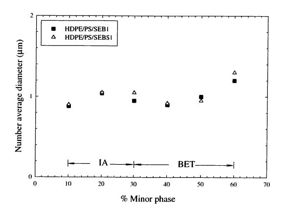
Figure 5.11 Pore size-composition relationship for HDPE/PS/SEBS1 and HDPE/PS/SEB1 blends.
