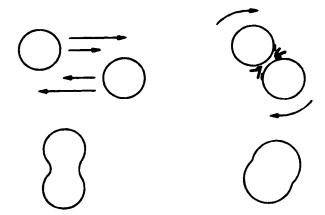
Figure 2.3 Idealized depiction of shear-induced coalescence of dispersed Newtonian droplets. The drops are brought close to each other by the shear field, and then the matrix film between the drops thins until the interface ruptures and coalescence occurs (Roland et al, 1984).
