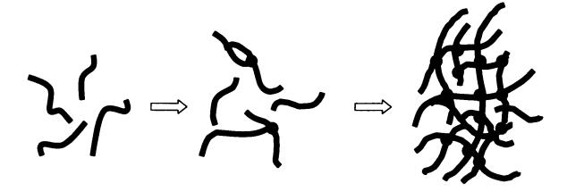
Figure 5.13 Schematic illustration of the development of co-continuity via thread-thread coalescence. This phenomenon occurs when the thread lifetime >> droplet lifetime (at low dispersed phase volume fraction) during melt mixing.
