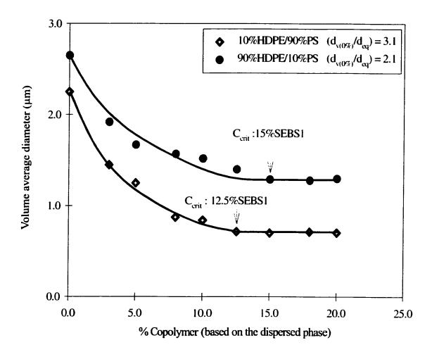
Figure 6.6.. Emulsification curves for 90%HDPE/10%PS and 90%PS/10%HDPE blends modified by SEBS1 triblock copolymer. The arrows indicate the critical concentration for interfacial saturation of the blend systems.
