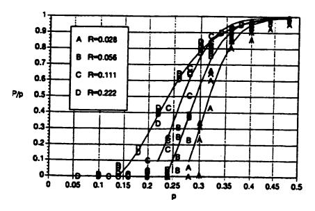
Figure 2.5 Effect of finite size on percolation: R is the ratio of inclusion to domain size in the percolation direction (Arends, 1992)
