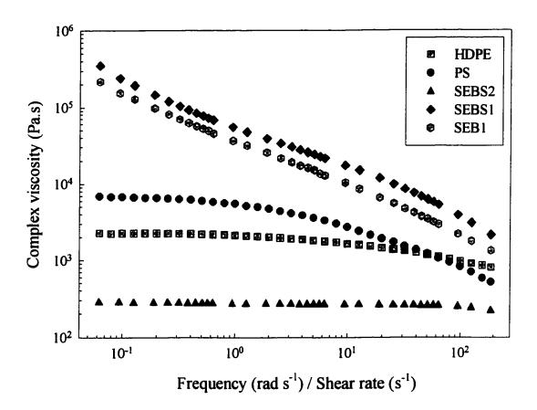
Figure 5.1 Complex viscosity-frequency/shear rate relationship for SEB1, SEBS1, SEBS2, HDPE and PS at 195°C.
