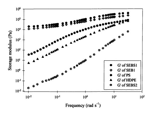
Figure 5.2 Storage modulus-frequency relationship for SEB1, SEBS1, SEBS2, HDPE and PS at 195°C.
