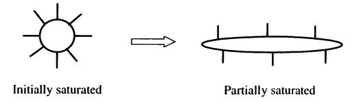
Figure 5.15 Schematic illustration of formation of co-continuity for the compatible ternary system. The saturated droplet saturated with interfacial modifier is deformed, and fresh interface is developed. If the time to emulsify the fresh interface is less than the time for breakup then this system also represents the case of droplet lifetime>thread lifetime (at low dispersed phase volume fraction).
