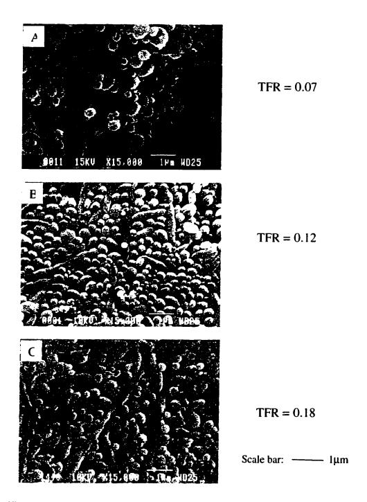
Figure 5.18 SEM photomicrographs of the dispersed HDPE phase and the corresponding TFR data after the matrix dissolution technique for a Type III system: (a) 5 HDPE/95 PS/20 SEBS1; (b) 10 HDPE/90 PS/20 SEBS1; and (c) 20 HDPE/80 PS/20 SEBS1.
