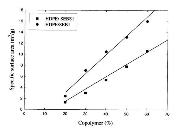
Figure 5.7 Dependence of specific surface area to copolymer amount for extracted HDPE/SEB1 and HDPE/SEBS1 blends.
