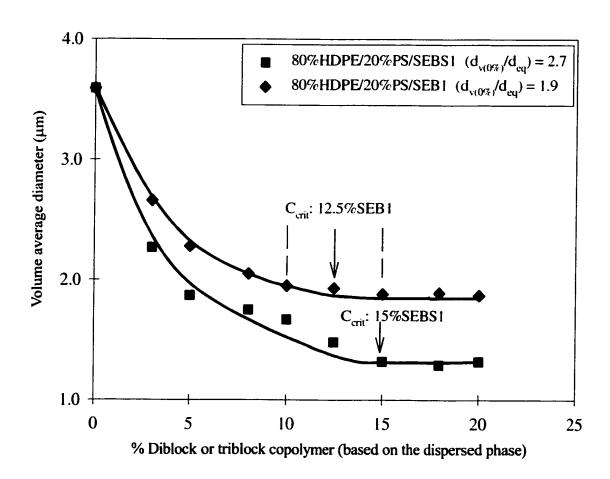
Figure 6.8b. The influence of the copolymer architecture (diblock vs triblock) on the emulsification of 80%HDPE/20%PS blend system.
