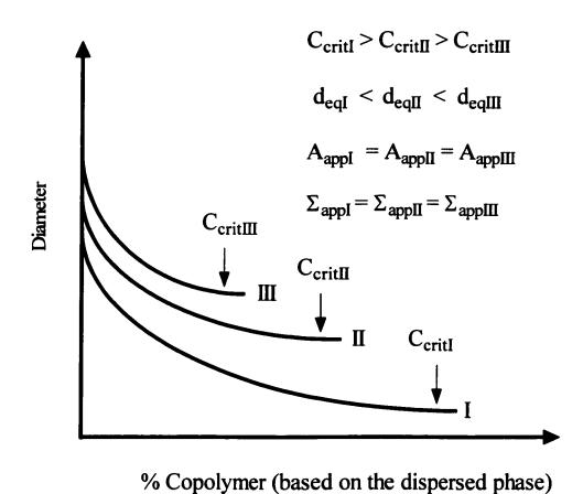
Figure 6.1c. Family of emulsification curves expected for the case where all the modifier migrates to the interface, but the modifier is ineffective at completely suppressing dynamic coalescence.
