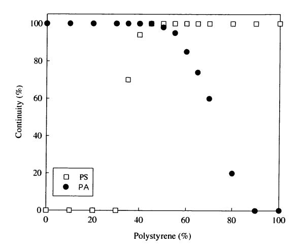
Figure 5 Continuity-composition relationship for compatibilized PA/PS blends.
