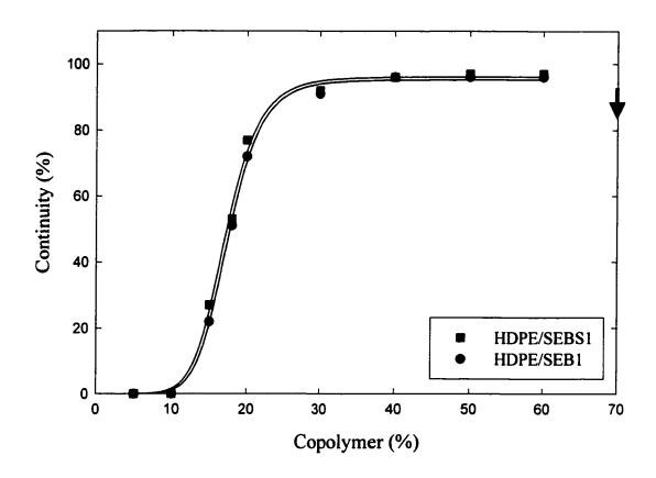
Figure 5.5. Continuity-composition relationship for HDPE/SEB1 and HDPE/SEBS1 blends. The arrow indicates the disintegration point for two blend systems.
