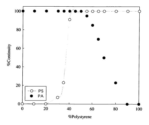
Figure 4 Continuity-composition relationship for non-compatibilized PA/PS blends
