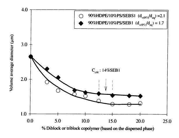
Figure 6.8a. The influence of the architecture of the copolymer (diblock vs triblock) on the emulsification of 90%HDPE/10%PS blend.
