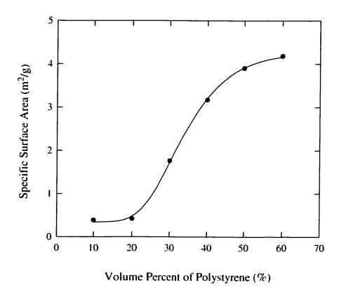
Figure 4.4. Effect of PS composition on the specific surface area for compatibilized blends. 20% SEBS interfacial modifier based on the minor phase was added.
