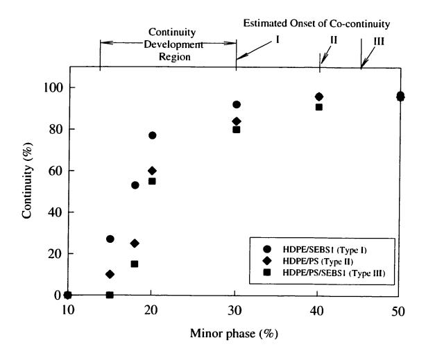
Figure 5.6b Expanded view showing the continuity/composition relationship for HDPE/SEBS1, HDPE/PS and HDPE/PS/SEBS1 blends.
