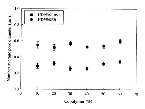
Figure 5.8 Pore size of extracted HDPE/SEB1 and HDPE/SEBS1 blends versus copolymer concentration.
