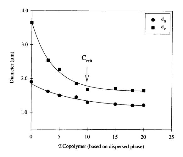
Figure 2 Emulsification curve for 10%PA/90%PS blend modified by SEBS-g-MA copolymer.
