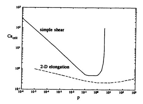
Figure 2. 1 Comparison of the effect of viscosity ratio on the critical capillary number in shear and elongational flows (Grace, 1982).
