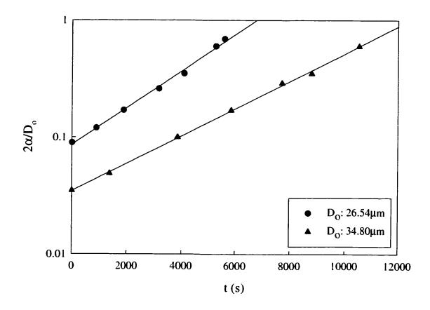
Figure 5.4 Relative distortion amplitude versus time for SEBS2 triblock copolymer imbedded in a HDPE matrix.
