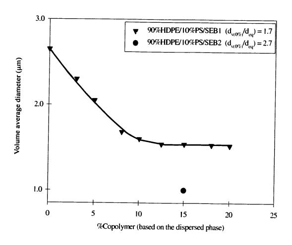
Figure 6.11. The influence of the chemical composition of diblock copolymer on the emulsification of HDPE/PS blends.
