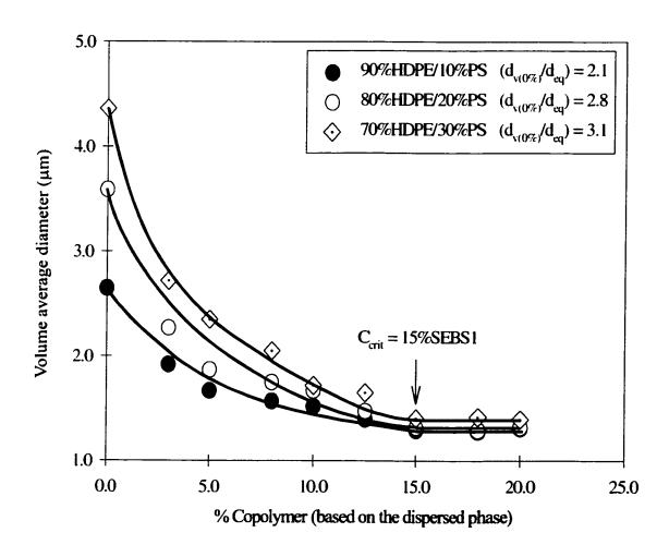
Figure 6.3b. A family of experimentally determined emulsification curves for 90%HDPE/10%PS, 80%HDPE/20%PS and 70%HDPE/30%PS.
