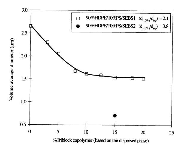
Figure 6.10. The influence of the chemical composition of triblock copolymer on the emulsification of HDPE/PS blends.
