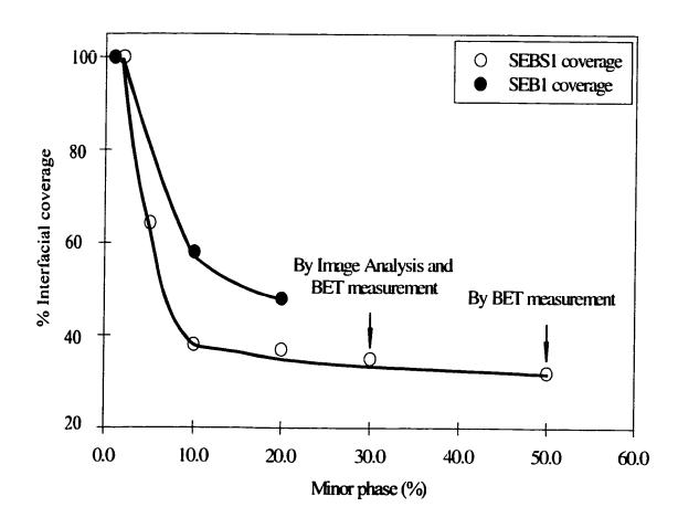
Figure 6.9. Interfacial coverage versus the dispersed phase concentration for blends compatibilized by diblock and triblock copolymer.
