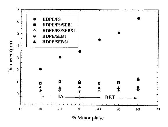
Figure 5.12 Pore size-composition relationship for HDPE/SEB1, HDPE/PS, HDPE/PS/SEB1, and HDPE/PS/SEBS1 blends.
