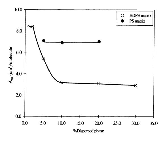
Figure 6.4. A<sub>app</sub> versus dispersed phase concentration for blends with both HDPE and PS as matrix.
