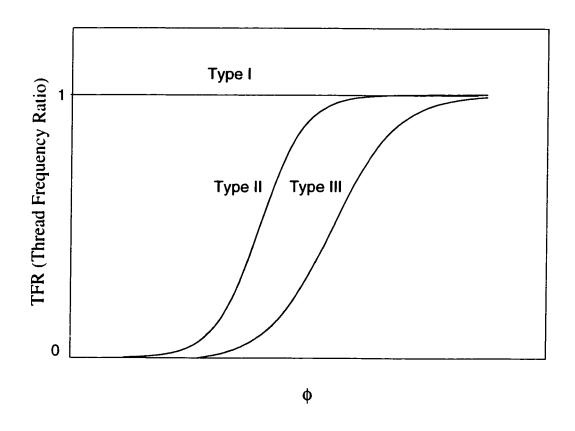
Figure 5.16 Schematic illustration of thread frequency ratio vs volume fraction for the three types of blend interfaces
