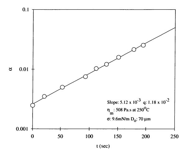
Figure 6 Relative distortion amplitude versus time for PA thread imbeded in a PS matrix.
