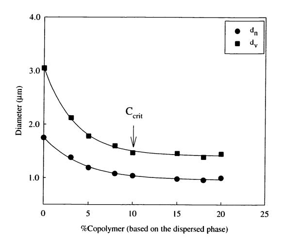
Figure 3 Emulsification curve for 90%PA/10%PS blend modified by SEBS-g-MA copolymer.
