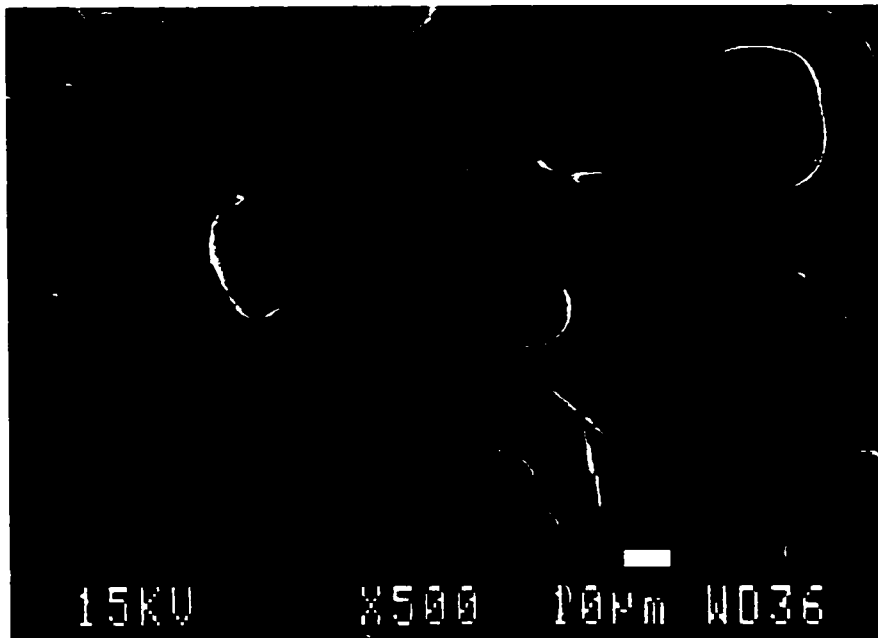
Figure 4.9 SEM cryofracture surface of PE1/TPS40 demonstrating excellent interfacial contact and mirror-like surface of the TPS phase.
