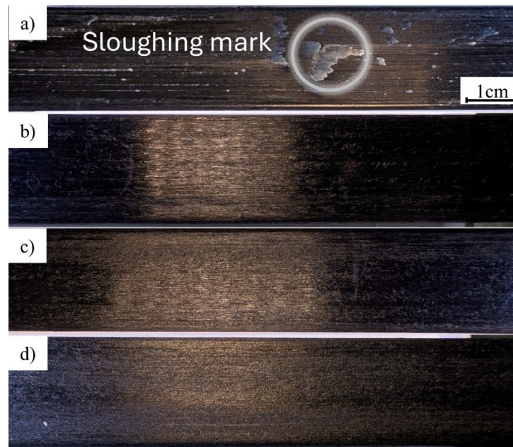
Figure 7.7 : Image of the surface of the pultruded bar, a) T-50-0 with a circled sloughing mark, b) T-50-15, c) T-500-15, d) T-1000-15
