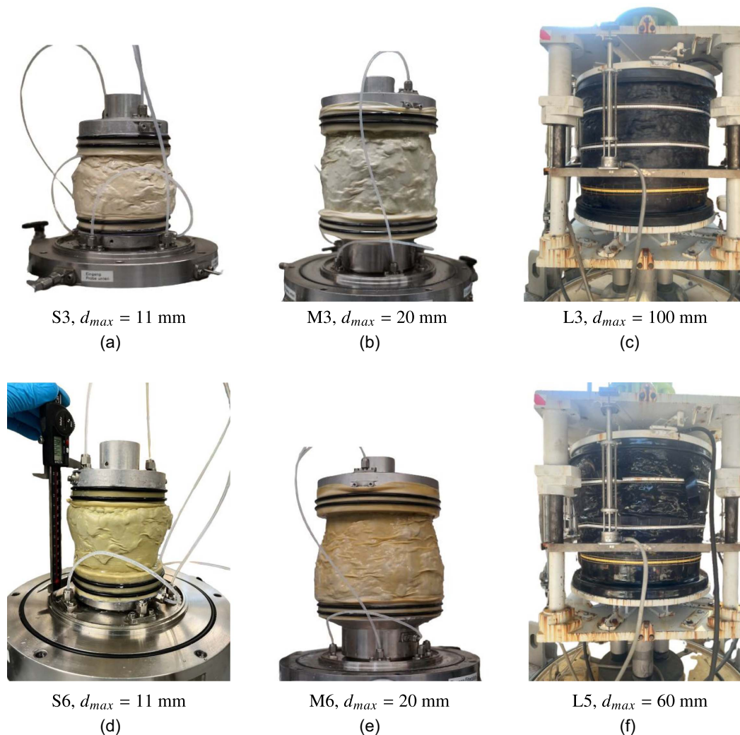
Fig. 16. Specimens after tests: (a and d) S specimen; (b and e) M specimen; and (c and f) L specimen. Panels (a)–(c) show \sigma'_3 = 100 kPa, and panels (d)–(f) show \sigma'_3 = 600 kPa.
