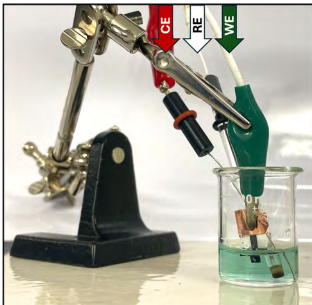
Figure 5.13 Voltammetry set-up for simple paper electrode including three separate electrodes (RE, WE (paper chip), CE) in the beaker containing the analyte (here, PYO solution, naturally blue)
