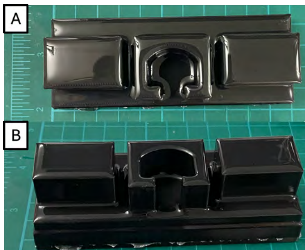
Figure 5.10 Top view (A) and side-view (B) of resulting PLA stamp coating by PDMS by pouring over PDMS.
