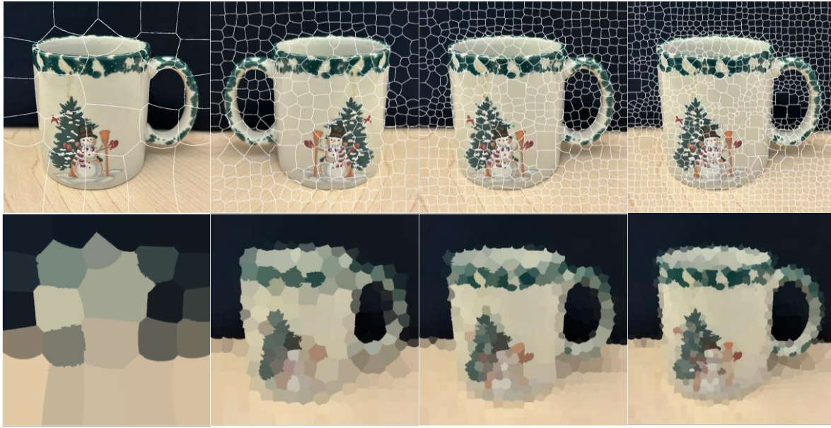
Figure 2.19 Top row: Results of using 25, 250, 500 and 1000 superpixels in the representations of Figure 2.18a). As before, the boundaries between superpixels are overlaid on the image for reference. Bottom row: Superpixel images.
