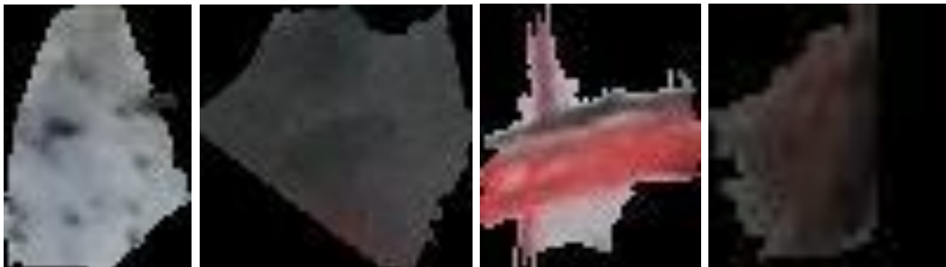
Figure 3.8 Result of classification. Superpixels from classes spodumene, gangue, marker and undetermined.
