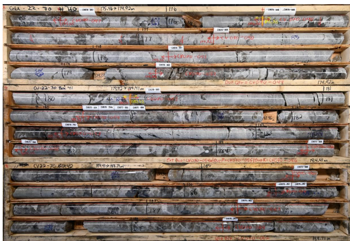
Figure 2.5 Drill cores stored in wooden boxes after collection from the site. The core box length is approximately 1,2 meters. Geologists have analyzed these cores visually and marked the location info on the cores. Example from a spodumene-bearing pegmatite of Patriot Battery Metals's Shaakichiuwaanaan project.
