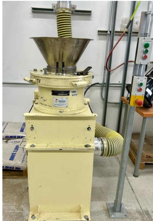
Figure 3.2 Metso Minerals Marcy cone crusher.
