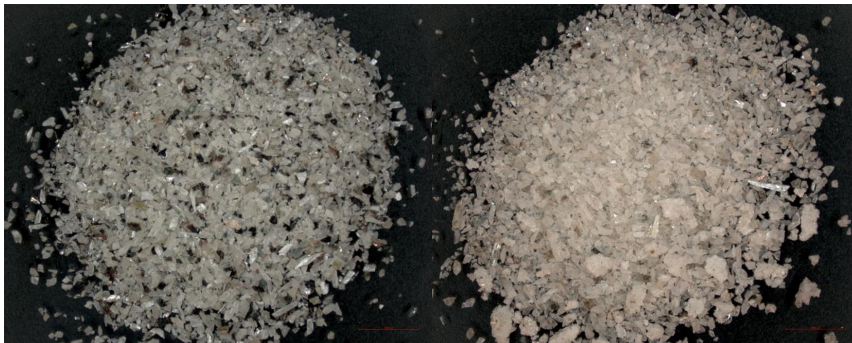
Figure 4.10 Sink (left) and float (right) fraction of fine particle (-0.6mm) centrifugation under the optical microscopy. 1 cm in the image represents 5000 \mu\text{m} in reality.
