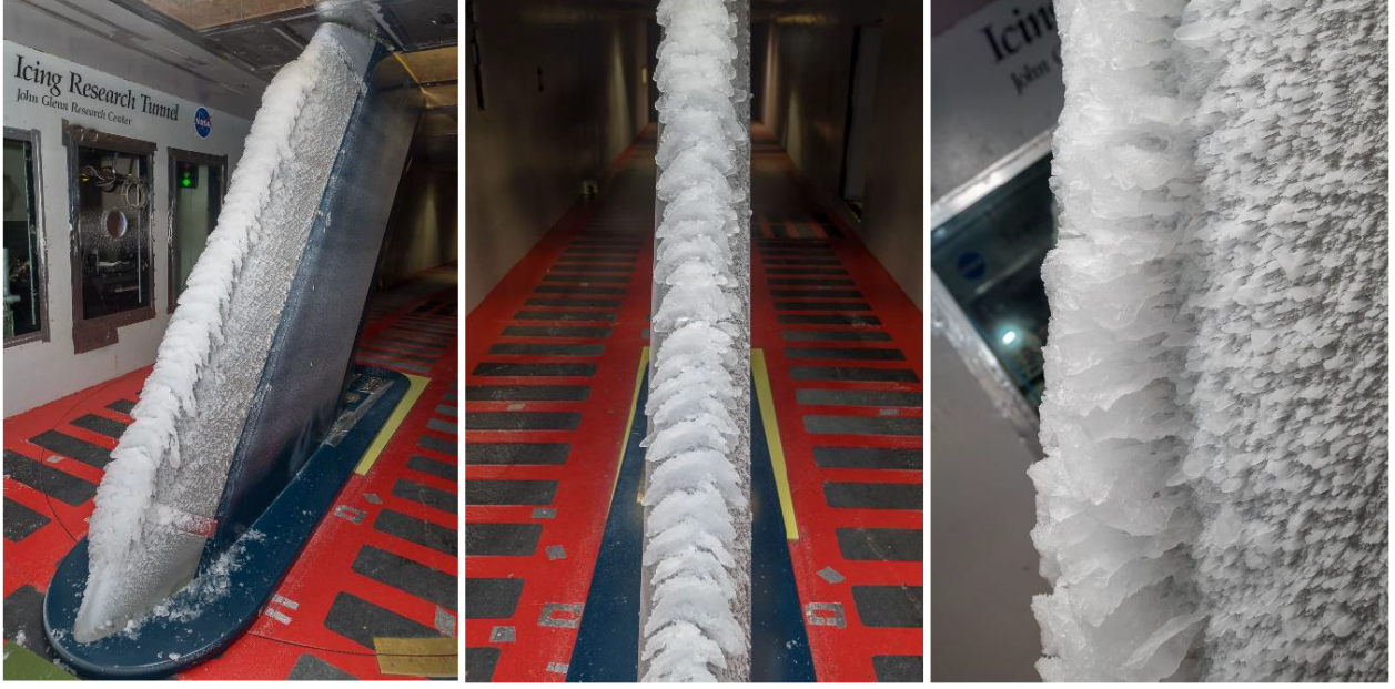
Figure 1.2 Scallop ice patterns observed on the CRM65 midspan model in the IRT for the 2 nd IPW. Image from [126].
