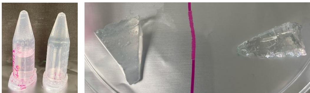
Figure 4.12 Gelation of sodium alginate (SA) and chitosan at 50:50 volume ratio SA:CMD, using EDC/NHS crosslinking chemistry. CMD was substituted with SA to display the versatility of our approach to produce clear and stable hydrogels.
