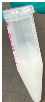
Figure 4.7 Formation of precipitates when the CHI solution (without addition of \text{NaHCO}_3 ) is mixed with CMD at pH 1-1.5.
