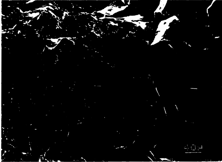
Figure 4.28 Interface of slow CCG region and fast fracture region of an CCG specimen solution treated at 1135°C and tested in air at 540°C.
