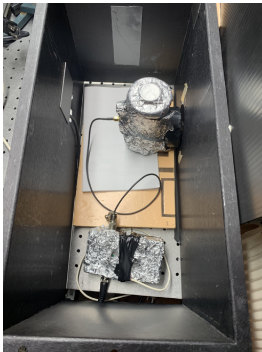
Figure 4.28 \text{O}_2(^1\Delta_g) detection setup: detector and signal pre-amplifier.
