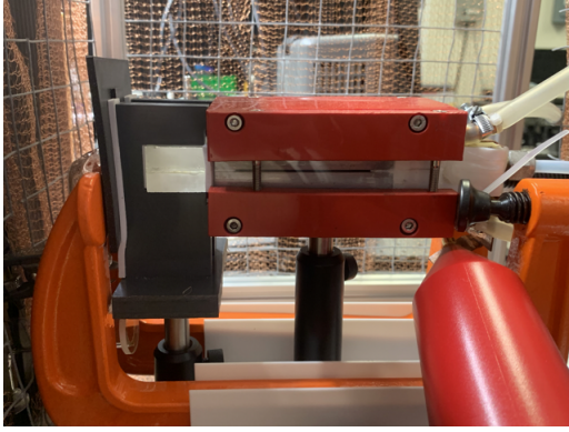
(a) Clamped APPJ and glass adapter
