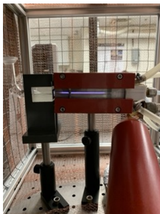
Figure 4.17 APPJ and collector adapter with a He gas mixture.
