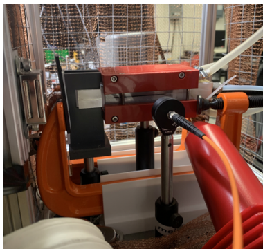
Figure 4.21 Bulk emission setup for the APPJ.
