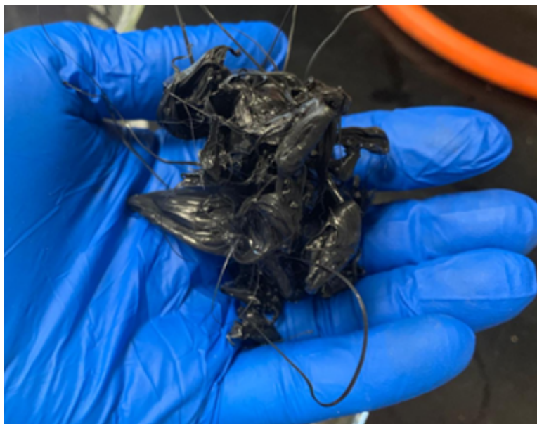
Figure 6.1 Agglomeration effect of large quantities. Due to the temperature, the polymer tends to agglomerate, forming agglomerates that make the kinetics difficult by reducing the surface contact with the solvent.
