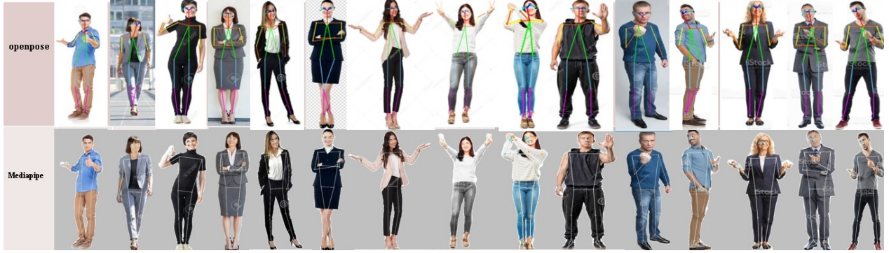
FIGURE 5.5 Qualitative comparison between OpenPose (top row) and MediaPipe (bottom row) on the same test images. MediaPipe yields a higher number of keypoints but requires more computation, whereas OpenPose provides structurally consistent poses with lower latency.
