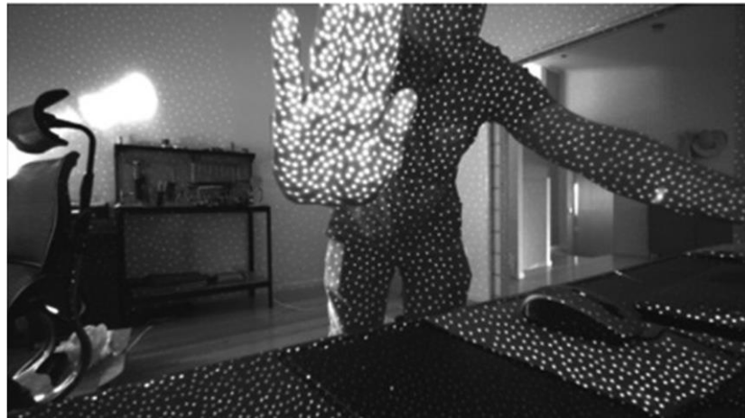
Figure 2.7 An example of a structured light method called the speckle pattern as used in the Kinect V1. It is a pseudo-random pattern of dots that helps for pattern matching to align features found in both images. (Clark et al., 2019)
