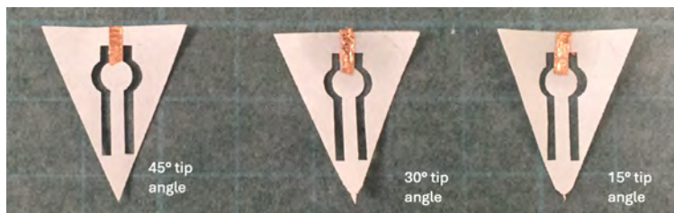
Figure 4.5 Photographs of the three fabricated \mu PADs with different tip angles ( 15^\circ , 30^\circ , and 45^\circ ).
