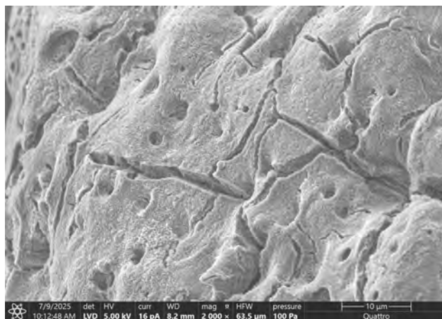
(a) ESEM image of a Whatman 2 paper tip with a 30^\circ tip angle, captured at \times 2000 magnification.
