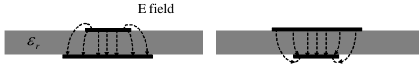
Figure 1.2: Electrical field plots on the A plane
