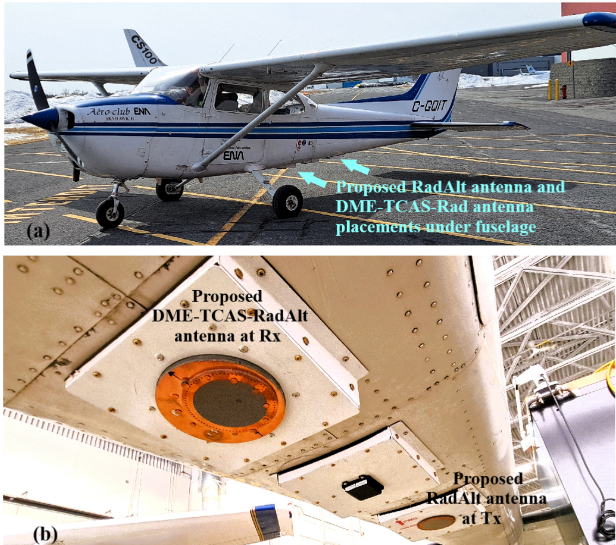
Figure 6.1 Proposed RadAlt and DME-TCAS-RadAlt antennas flight testing aircraft and placements (a) Antennas placement under aircraft fuselage, (b) Bottom view of antennas placement under aircraft fuselage.
