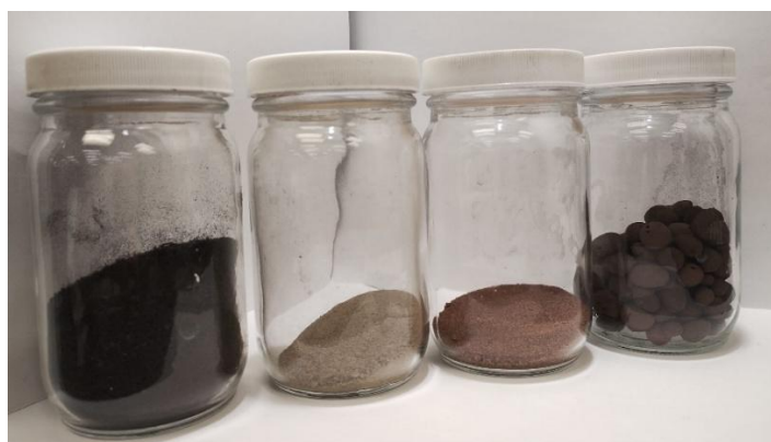
Figure 5.2. Four native materials as mineralizing agents: soil, beige sand, red sand, and clay (left to right). Gravel was also initially tested, but due to its limited performance, it was not included in further analyses.
