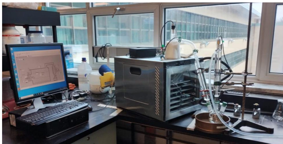
Figure 3.2. First generation atmospheric water harvesting laboratory prototype
