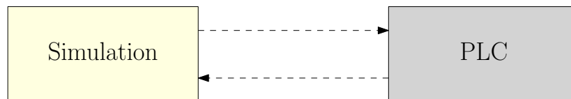
Figure 3.6 A Modbus server in the MATLAB simulation communicates process values directly with the BLC PLC
