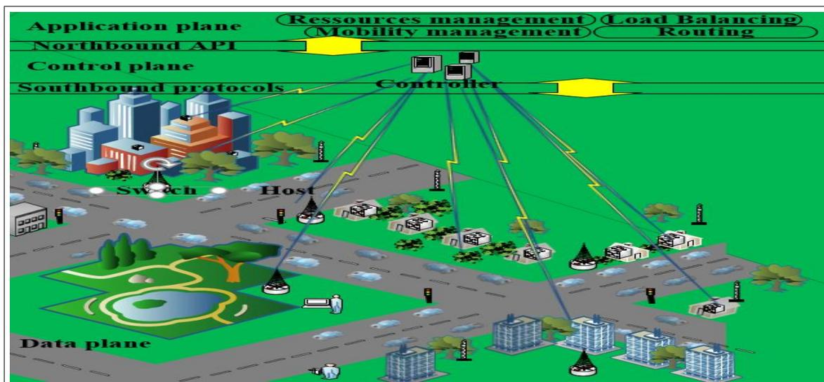
Figure 6.1 SDN architecture in Smart City Environment
