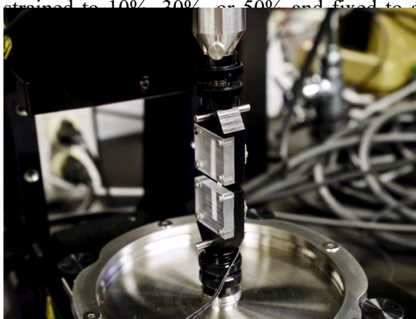
Figure B.2 Electrical tensile tester loaded with PEDOT:PSS sample.
