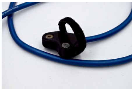
Figure B.12 Steel electrodes and cable used to record EDA.
