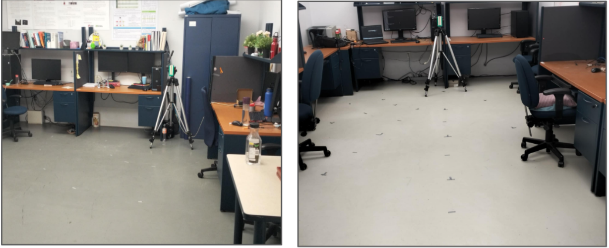
FIGURE 4.6 Data acquisition environments : LAB1 (right), LAB2 (left). LAB1 has an higher clutter levels, with additional interference caused by furniture, walls, and electromagnetic reflections. The second environment (LAB2) exhibited lower clutter levels. Ventilation systems, and other active equipment contributed additional noise.
