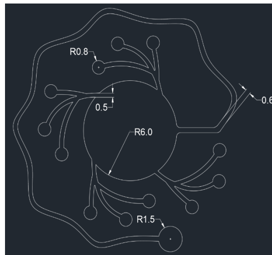
Figure S4. Custom-designed microfluidic layout for sweat collection and neurotransmitter monitoring (dimensions in mm). The design features a central circular chamber (radius: 6.0 mm) connected to twelve inlet channels and a single outlet channel, enabling efficient fluid distribution and collection.
