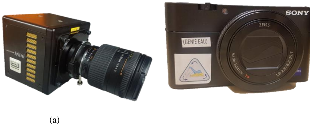
Figure 3.2 - (a) The FASTCAM Mini WX100 placed above the tank. (b) The camera Vixia HF S200 camera placed in front of the tank
