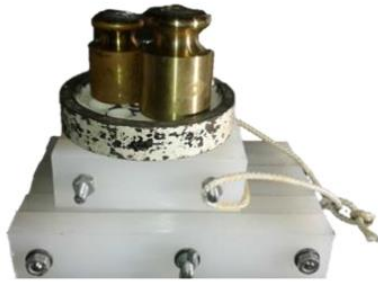
Fig. 2. Polypropylene strips and weights used for measuring static friction coefficient.
