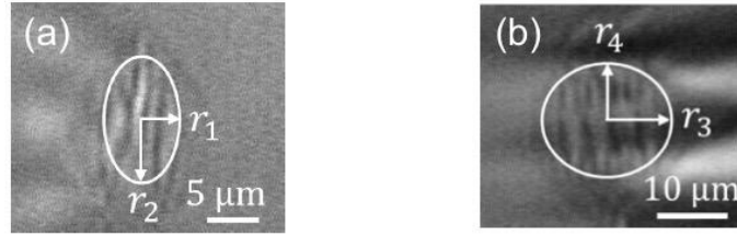
Figure A.4 Side views of (a) PO-WGs (with dot) of dot-Bragg grating, and (b) DO-WGs of line-Bragg grating.
