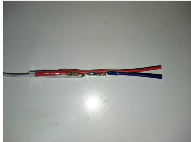
(b) Heat-shrink insulation over resistor and leads.
