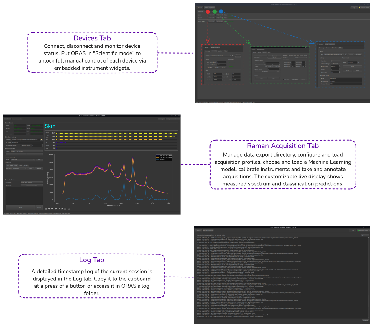
FIGURE 4.16 Main GUI of the ORAS software, showing the three primary tabs : Devices for instrument connection and status monitoring, Raman Acquisition for configuring and taking spectral measurements with live display and ML predictions, and Log for accessing a timestamped session history.
