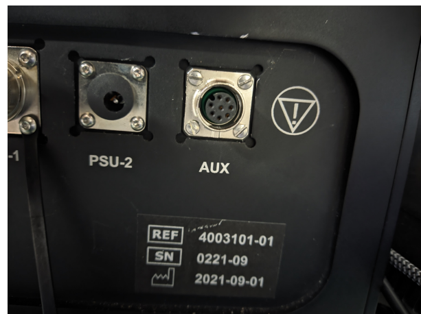
(b) Panel connector mounted to the rear of the Sentry unit.
