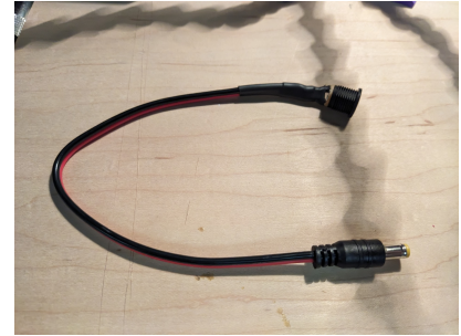
(c) Assembled barrel jack connector prior to installation.
