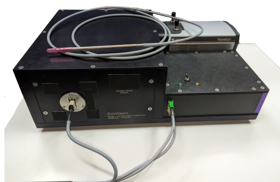
(d) The LRS-mini system, a compact and portable variant designed for laboratory-based testing and development.
