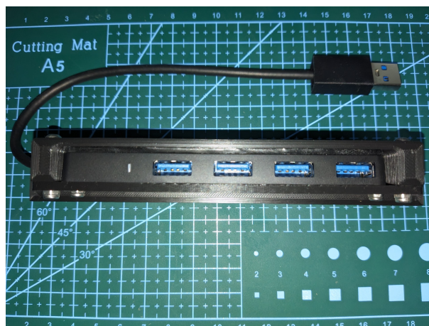
(b) USB hub secured in place within the 3D-printed fixture using adhesive tape.
