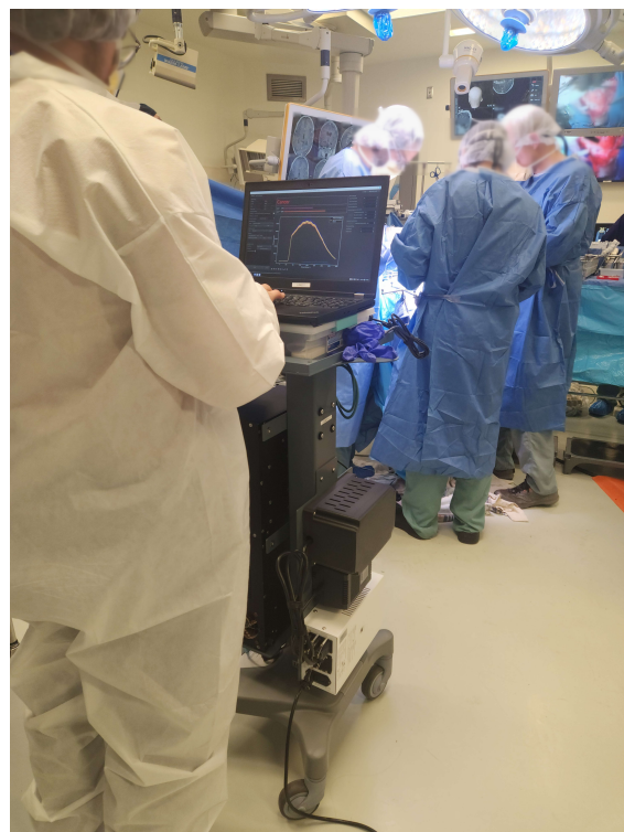
(b) The LRS in use during an intraoperative brain measurement in the operating room.
