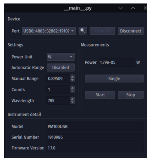
FIGURE 4.15 (a) Example of the Powermeter class from the tpm_control module within a Python shell. (b) Screenshot of the Thorlabs powermeter control widget in a standalone Qt application.
