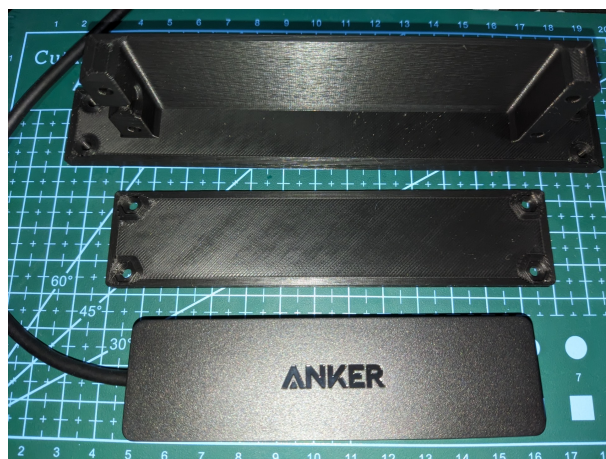
(a) USB hub next to the 3D-printed bracket prior to assembly.
