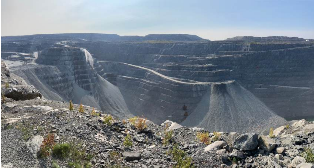
Figure 2.10 Real case scenario of end-push dumping during pit back-filling (Canada) after Garcia-Torres et al. (2024).
