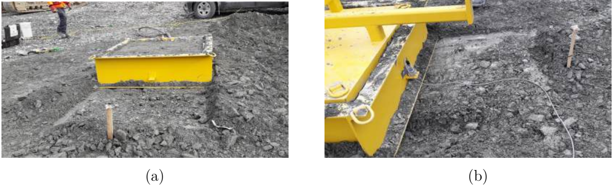
Figure 3.20 Large shear strain attained beyond h \geq 40 \text{ cm} : (a) back view; (b) side view.
