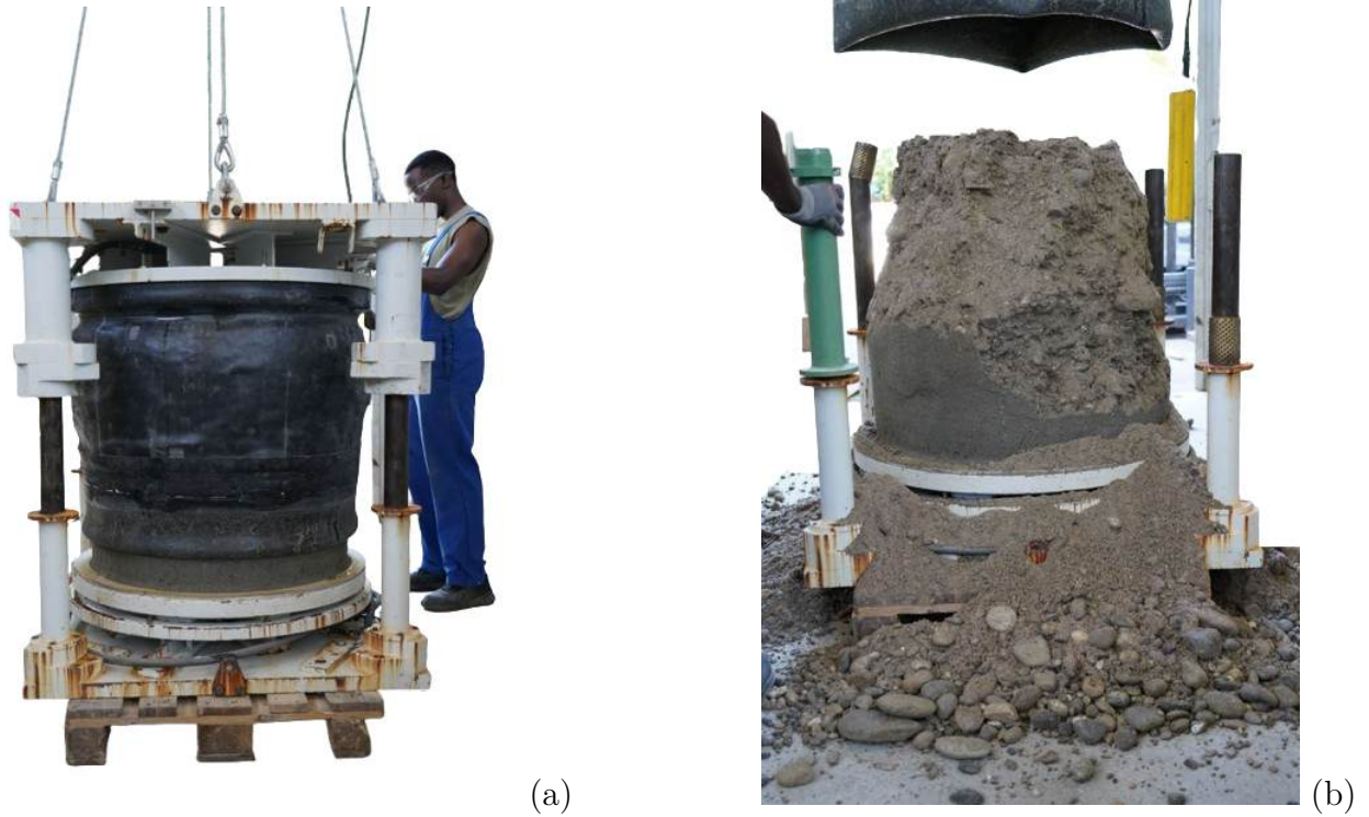
Figure 3.24 L2 ( D = 800 mm) specimens after testing: (a) removing the membrane; (b) view of alluvial gravels in the specimen.
