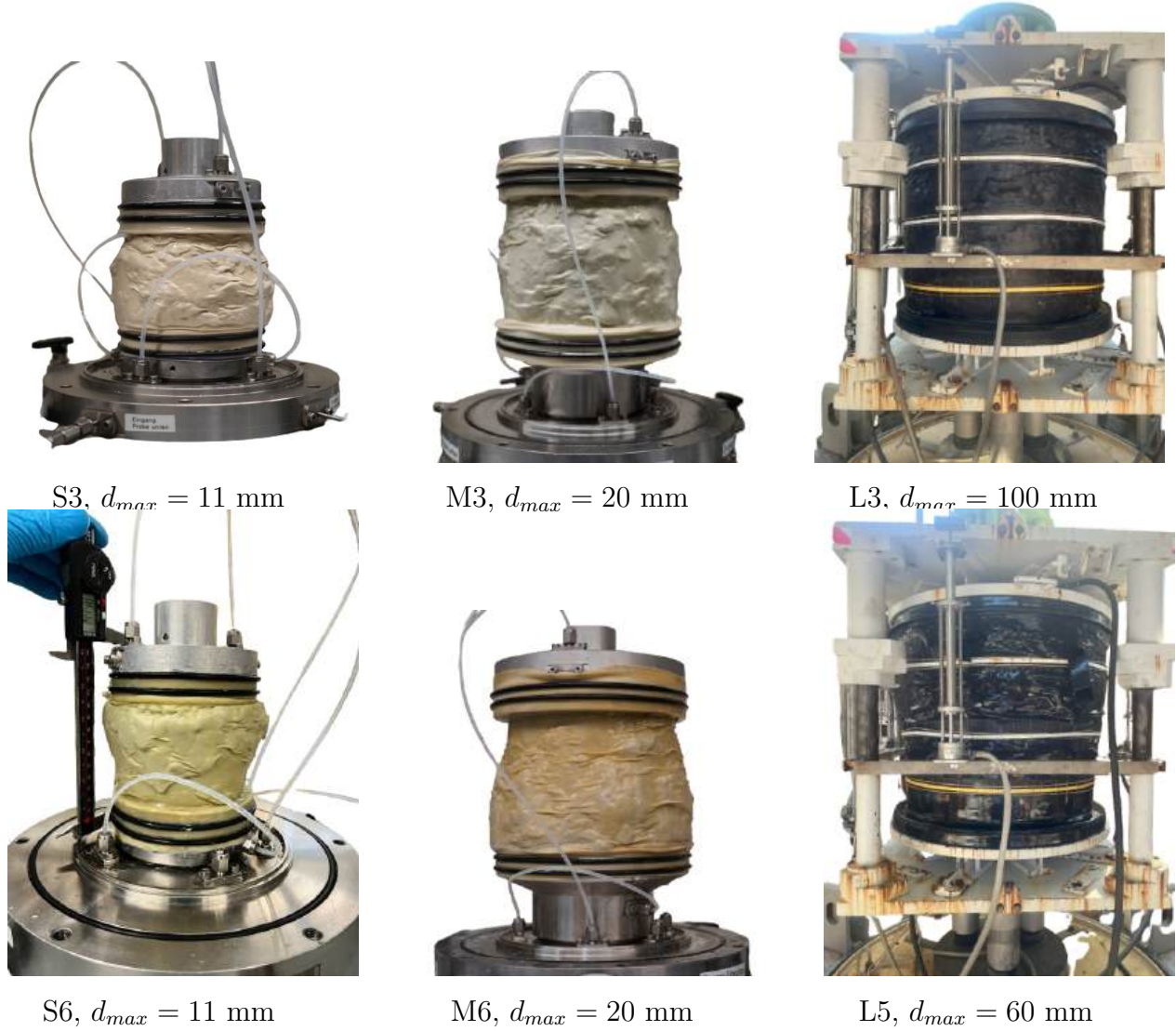
Figure 6.15 Sample photos after tests: from left to right S, M & L samples, and top to bottom \sigma'_3 = 100 kPa & 600 kPa, respectively.
