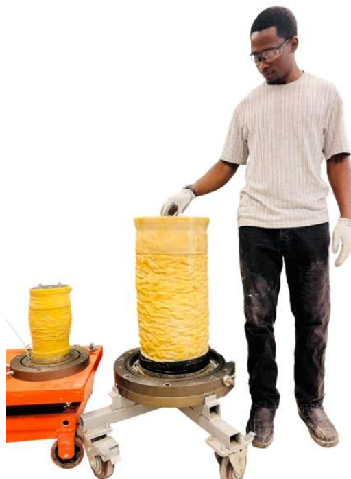
Figure 3.14 Photos displaying M1 ( D=150\text{mm} ) and L1 ( D=300\text{mm} ) specimens after test.
