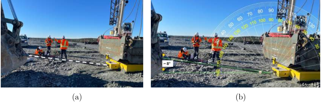
Figure 3.19 In-situ DST shearing: (a) showcase of the test under F_v = 30t ; (b) online measurement of the inclination angle for data correction.
