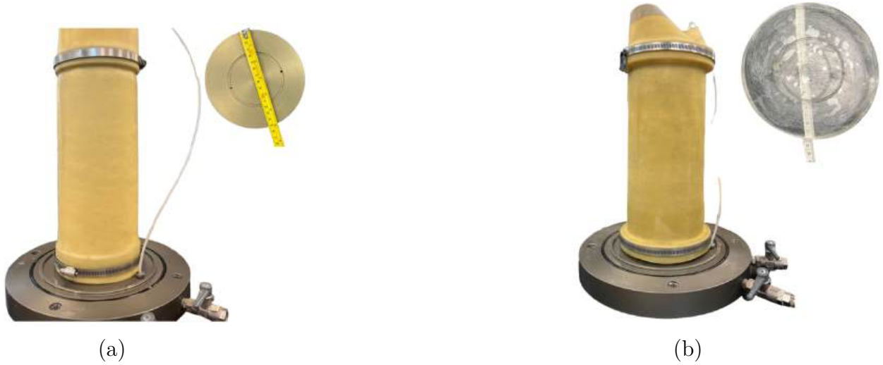
Figure 3.15 Photos of M1 specimens before testing: (a) with standard cap and base; (b) with enlarged-lubricated cap and base.
