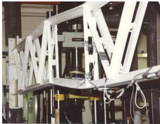
Figure 2-8 : Deformation in the Vierendeel special segment (Basha & Goel, 1994)
